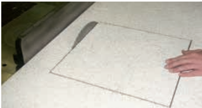
Cutting out of the opening/cover tile from the reverse side of the tile.
